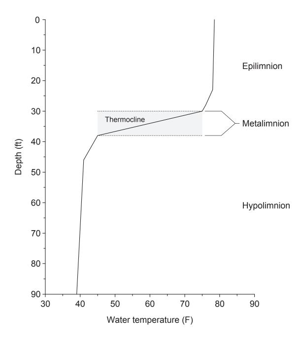
Figure 4.-Typical thermal stratification of a lake (adapted from Wetzel 1975).
